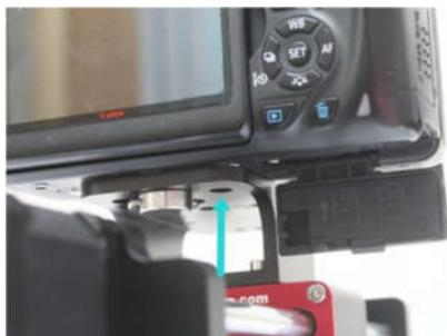
Of course, most cameras be installed in the middle, Because of the slim base, you can change battery without taking the camera off. And you can install camera in the hole beside to adjust for battery changing.
